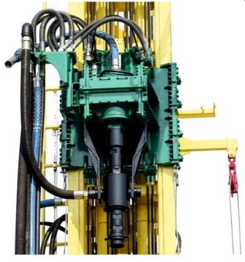
reduction and oil bath lubrica?on type gearbox along with top air entry and bottom entry mud swivel having ID: 90 mm spindle with thread connec?on of API 6 5/8 Reg driven by two hydraulic motor.
